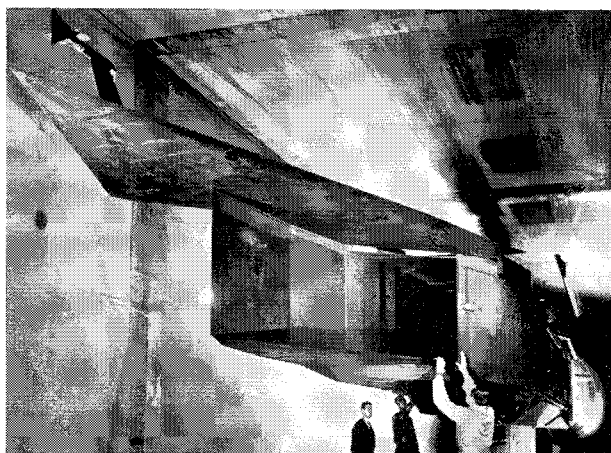
Fig. 9 One-third flow scale inlet model test at AEDC.
